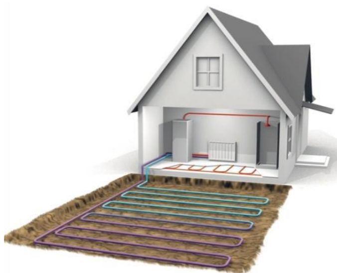
FIGURE 31: GEOTHERMAL HP WITH HORIZONTAL INSTALLATION (SOURCE: THERMIA HEAT PUMPS)
